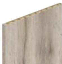
Side panel 32 mm thick, two sides finished with TopLaminate, one long visible side finished with ABS/PP*
